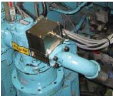
MetalSCAN installed on a GE1.5 turbine
